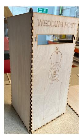
Using a Mitre Bond glue, (Glue + Activator) soft assemble the front panel and the Left panel together.
