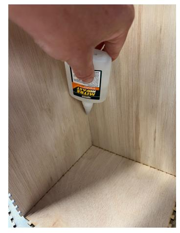
Once the Floor, Front, Left and Right Panels along with the Roof is all assembled, its very easy to glue the back panel on.
