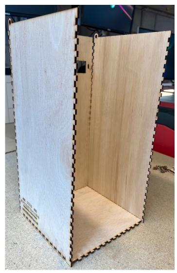
Now place the right panel against the face & floor panel. Before gluing the panels, place the lid on top with the hinges in the holes.
